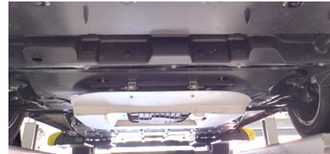
Trial mounting activity in pilot phase showing low position of the vehicle pad and EM shield
